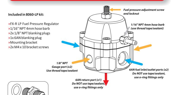
**Caution!!!** The fuel inlet/outlet and return ports use 6AN ORB (O-Ring Boss) type fittings and adapters. Be aware that they are NOT pipe threads and do NOT require thread sealant - they are reliant on the o-rings for a positive seal. Please ensure that you use ORB-type fittings.
